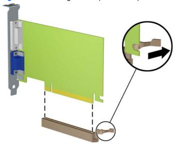
Figure 6-20 Removing a PCI Express x16 Expansion Card
